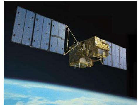
GOSAT observes infrared light reflected and emitted from the earth's surface and the atmosphere. Column abundances of CO<sub>2</sub> and CH<sub>4</sub> are retrieved from the observed spectra. The mixing ratio of the target gas species is expressed as column-averaged dry air mole fraction above an observed unit surface area of 10.5 km.
