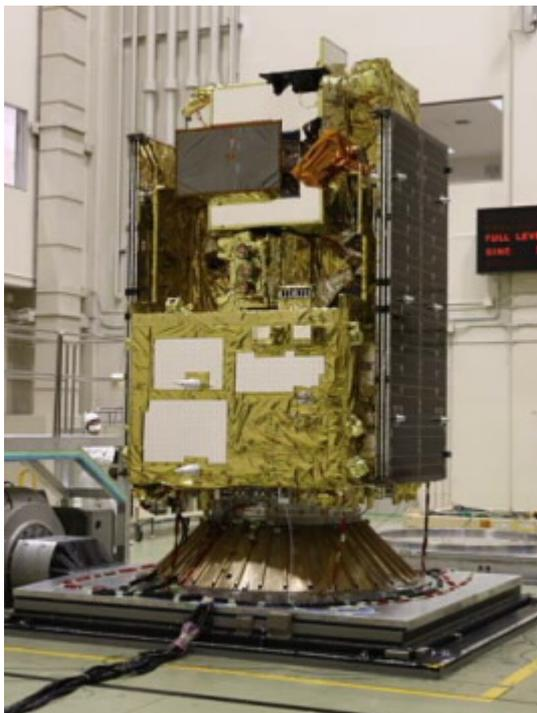
**Fig. 2. Vibration test**
