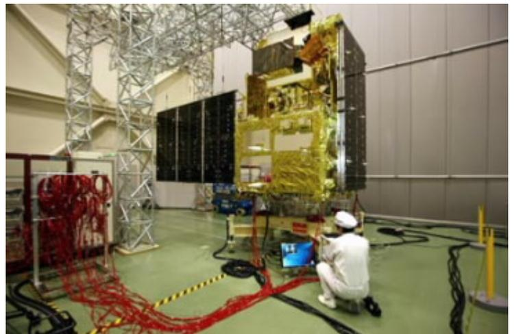
**Fig. 3. Solar paddle deployment shock test**
