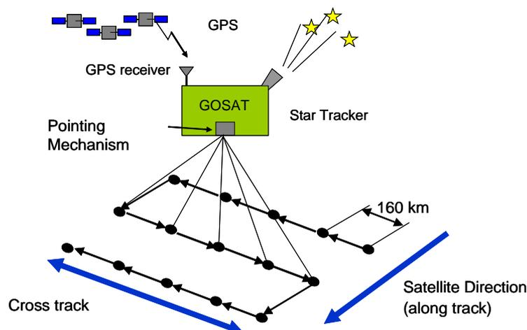
Fig. 10. The concept of attitude control and ground pointing.
