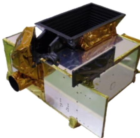
**Fig. 4. The proto-flight model of TANSO-FTS**
