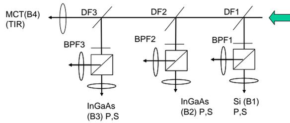
Fig. 6. The band separation optics and the detectors.
