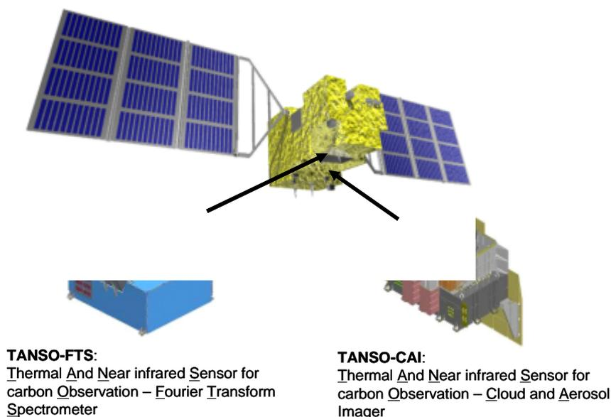
Fig. 1. The GOSAT satellite and sensors.
