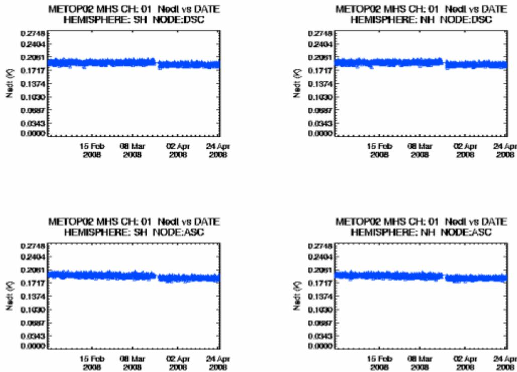
**Figure 6:** Time series of Metop-A MHS Channel 1 NEDT for 25 January to 25 April 2008. The four plots are divided into Northern (Southern) Hemisphere region on the right (left), and ascending (descending) node on the bottom (top).
