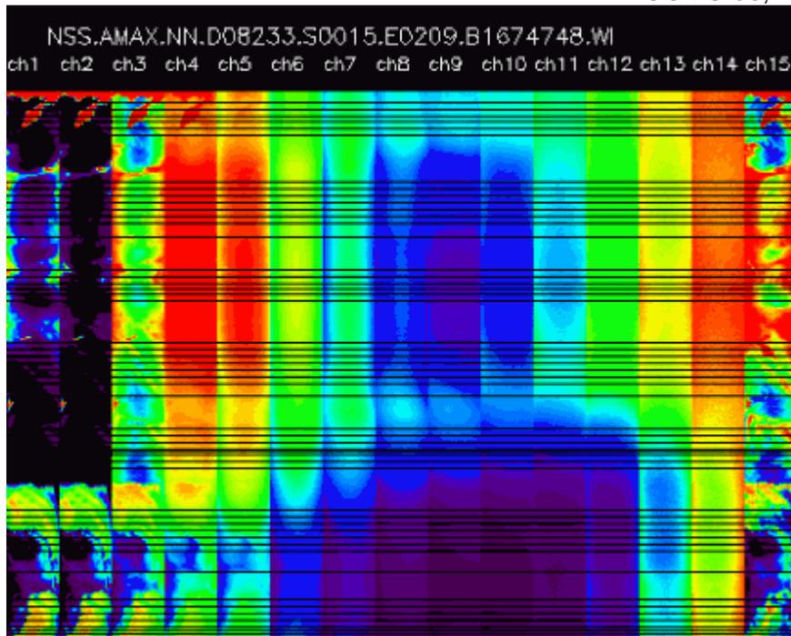
**Figure 8:** One orbit AMSU-A image for all 15 channels on 20 August 2008 from NOAA-18 AMSUA. There are many dropped lines due to the instrument noise problem.
