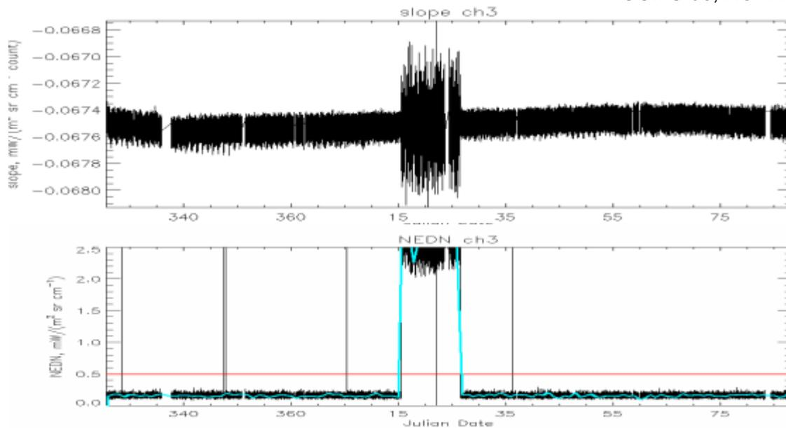
**Figure 7:** Time series of calibration coefficients and NEDN for channel 3 of Metop-A HIRS. The red line is the designed specific NEDN value while the blue line is daily-mean NEDN value.
