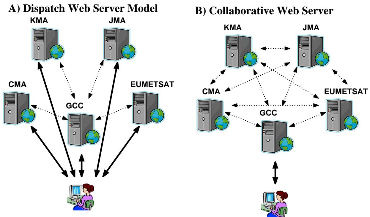
**Figure 3:** Dispatch (A) and collaborative (B) web server models for controlling the flow of information to users looking for IPM information and data.
