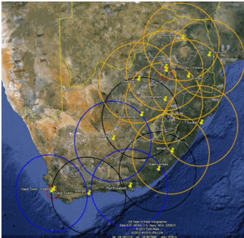
Figure 2: SAWS radar network. Blue: C-band Black: S-band (planned) Orange: S-band (in operations) Red: X-band radar at the major airports, not operational
