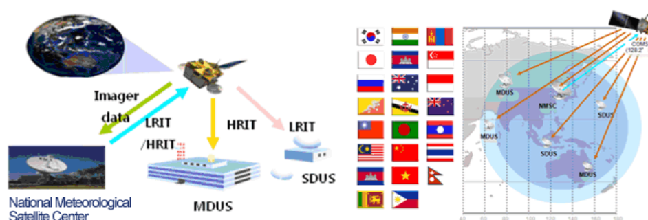
Figure 2.2: Concept of MI H/LRIT direct broadcasting
