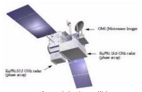
Administration (NASA) and JAXA. The accurate measurement of precipitation will be achieved by the Dual-frequency Precipitation Radar (DPR) installed on the GPM core satellite. The DPR on the GPM core satellite is being developed by JAXA and National Institute of Information and Communications Technology (NICT).
