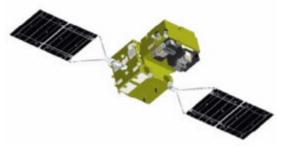
The first generation of GCOM-C (called GCOM-C1) is scheduled to be launched in JFY2015 or later. Its orbit will be sun-synchronous with 798km altitude (over the equator), 98.6 degrees inclination and 10:30 local time of descending node.
