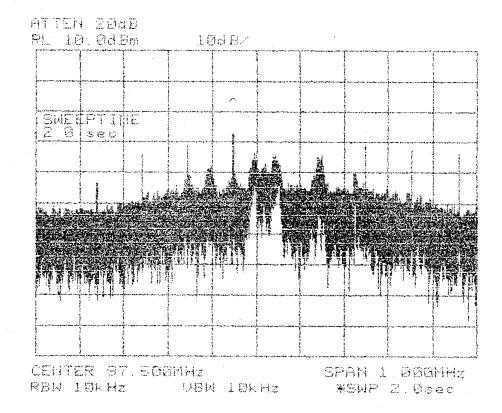
FY-2 Interference Spectrum of DCP UHF Band (The impulse interval is about 200ms)
