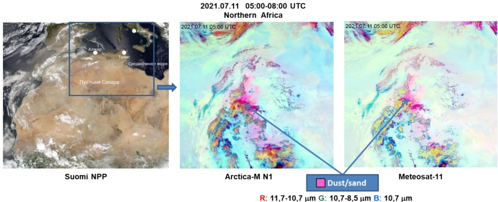
The transport of dust (sand) particles is clearly traced based on satellite data presented on this slide. To detect clouds of dust (sand), combinations of specific satellite channels are used in wavelength ranges that are sensitive to certain fractions, in this case to dust (sand) particles. In the images, dust is depicted in pinkish colors.
