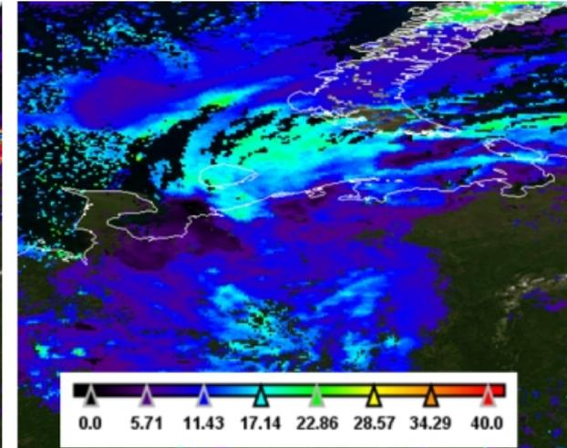
Cloud particle effective radius,  $\mu\text{m}$
