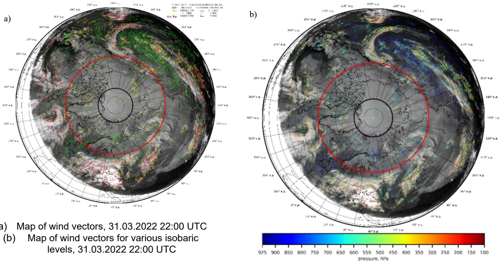
MSU-GS/A Arctica-M N1 data received with high frequency (during the western and eastern passes) can be considered as unique for identification of atmospheric motion vectors (speed and direction at different levels) in the area. For the first time maps of wind vectors for the Arctic region and neighbouring territories are prepared with a high temporal resolution – every 15 minutes.
