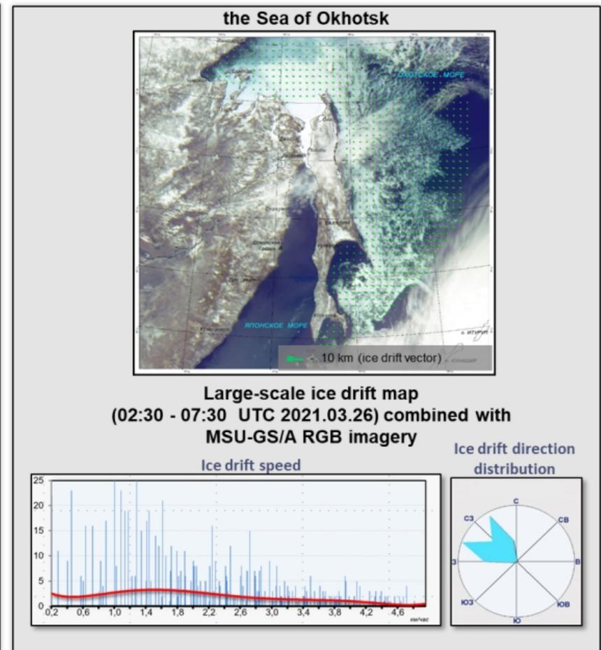
MSU-GS/A Arctica-M data enables to track large-scale ice drift in a short time interval and determine areas of intense ice drift at a speed of at least 1 km/h, which pose a particular danger to shipping and maritime industries.
