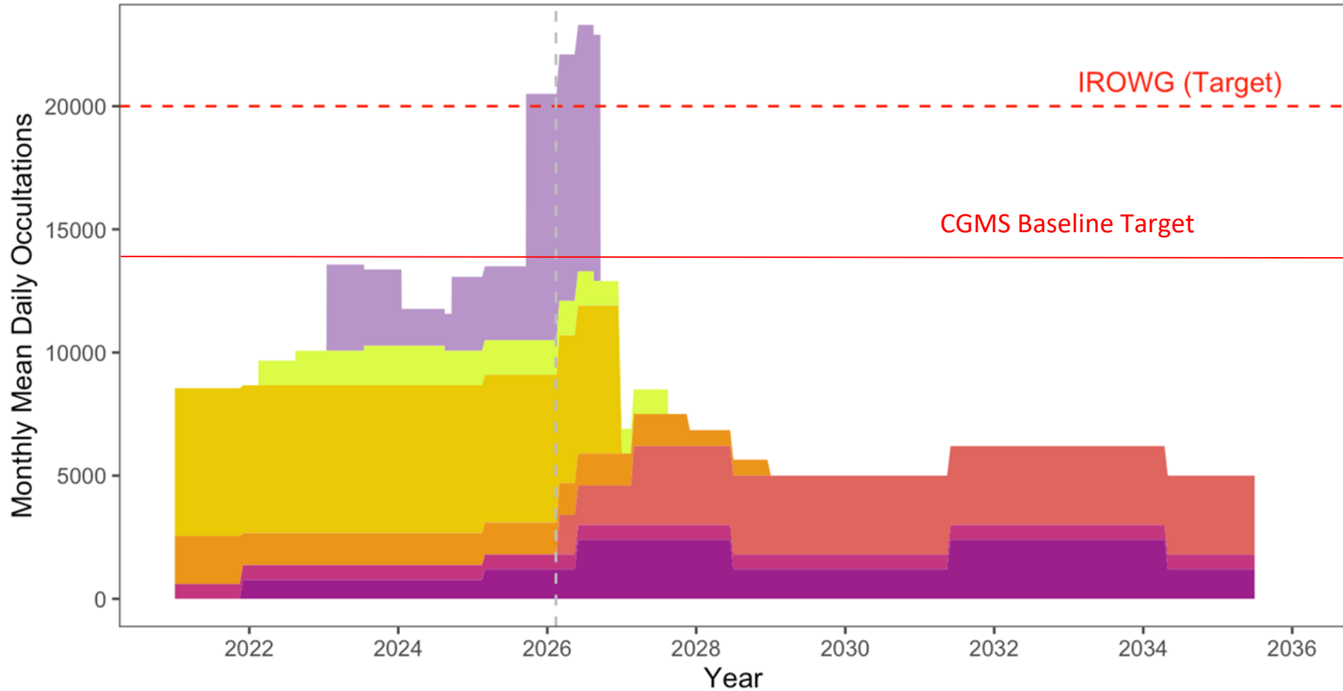
Monthly Mean Daily RO Numbers (NRT)* (as available today or from mission requirements)
