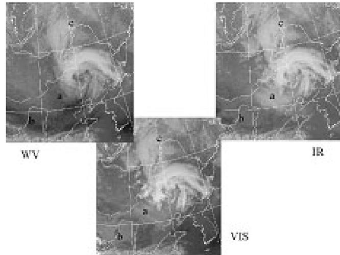
**Figure 2.** WV, IR and VIS images for a dust target (a: dust-storm; b: open region; c: cirrus)
