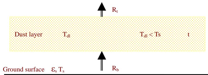
**Figure3** Mechanisms explaining the depression of thermal infrared radiance outgoing to space in the presence of a dust layer over land
