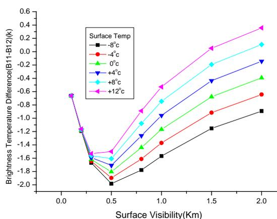
**Figure 1. The relationship between surface visibility and temperature differences a function of ground surface temperatures for middle latitude winter atmosphere**
