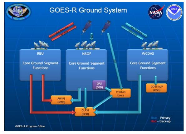
The ground system is composed of computers which control the satellite and process the satellite's data into products scientists can use the antenna system for command and data acquisition.
