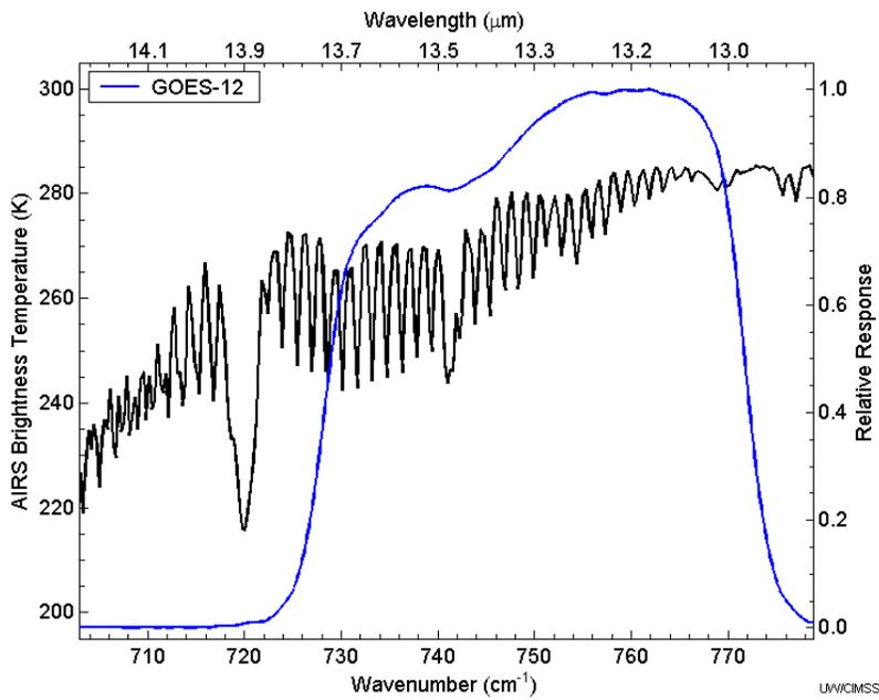
Figure 5. 13 μm band GOES-12 spectral response function plotted with representative AIRS brightness temperature spectrum.
