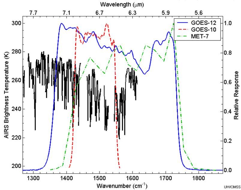
Figure 2. 6  $\mu\text{m}$  band spectral response functions plotted with representative AIRS brightness temperature spectrum. GOES-9 has similar spectral coverage to GOES-10 and Meteosat-5 has similar spectral coverage to Meteosat-7. Note the large percentage of SRF not covered on the shortwave side by AIRS data for the wider responses of GOES-12 and Meteosat.
