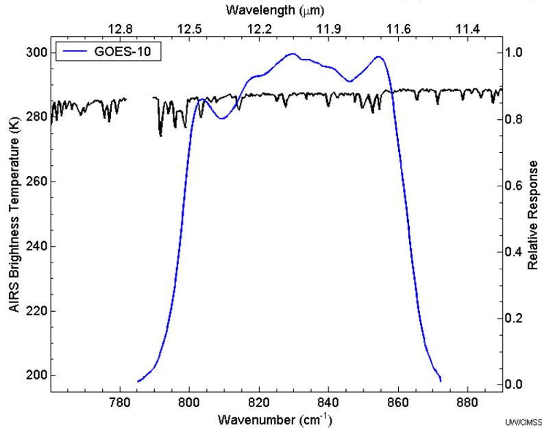
Figure 4. 12 μm band GOES-10 spectral response function plotted with representative AIRS brightness temperature spectrum. GOES-9 has similar spectral coverage to GOES-10.
