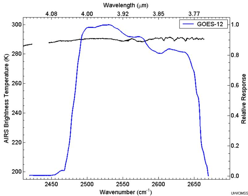
Figure 1. 3.9  $\mu\text{m}$  band GOES-12 spectral response function plotted with representative AIRS brightness temperature spectrum. GOES-9 and GOES-10 have similar spectral coverage. Note that on the shortwave side, AIRS coverage ceases very close to the end of GOES spectral coverage.
