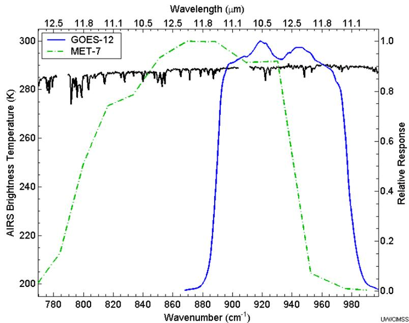
Figure 3. 11  $\mu\text{m}$  band spectral response functions plotted with representative AIRS brightness temperature spectrum. GOES-9 and -10 have similar spectral coverage to GOES-12 and Meteosat-5 has similar spectral coverage to Meteosat-7.
