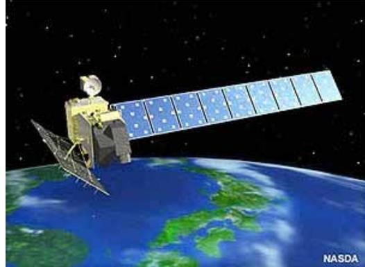
ALOS is one of the world's largest earth observation satellites whose function is to collect global and high resolution land observation data. Because of the large increase of observation data it will be transmitted to EOC via both [DRTS](#) and as a direct downlink. In this way observation data can be rapidly acquired by EOC from all areas.
