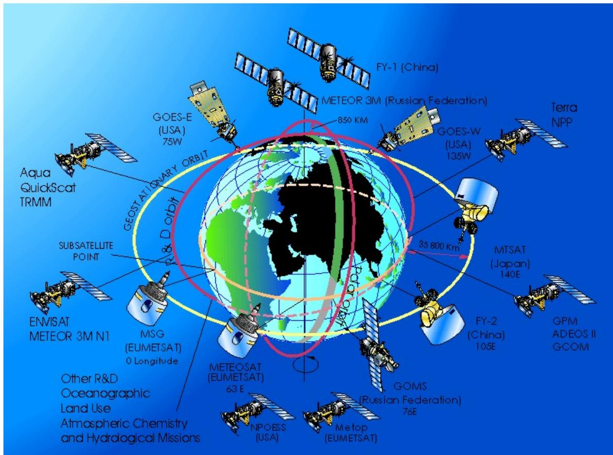
Figure 1 – Space-based component of the Global Observing System at CM-3
