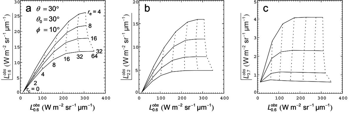
Figure 1 Comparison of 1.6-, 2.2-, and 3.7- $\mu\text{m}$  radiances as a function of cloud optical thickness (0, 2, 4, 8, 16, 32, 64) and effective radius (4, 8, 16, 32) with the angular variables of the satellite zenith angle ( $\theta$ ) =  $30^\circ$ , the solar zenith angle ( $\theta_0$ ) =  $30^\circ$ , and the azimuth angle of the satellite relative to the sun ( $\phi$ ) =  $10^\circ$ .
