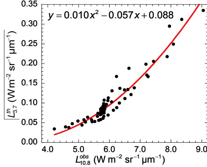
Figure 2 Sensitivity of 3.7- $\mu\text{m}$  thermal radiances to 10.8- $\mu\text{m}$  satellite-received radiances for the clouds with a variety of cloud optical thickness (0 to 64) and effective radius (0 to 32  $\mu\text{m}$ ) under diverse cloud top temperature and ground temperature. The solid line is the 2<sup>nd</sup>-order polynomial regression line of the plots.
