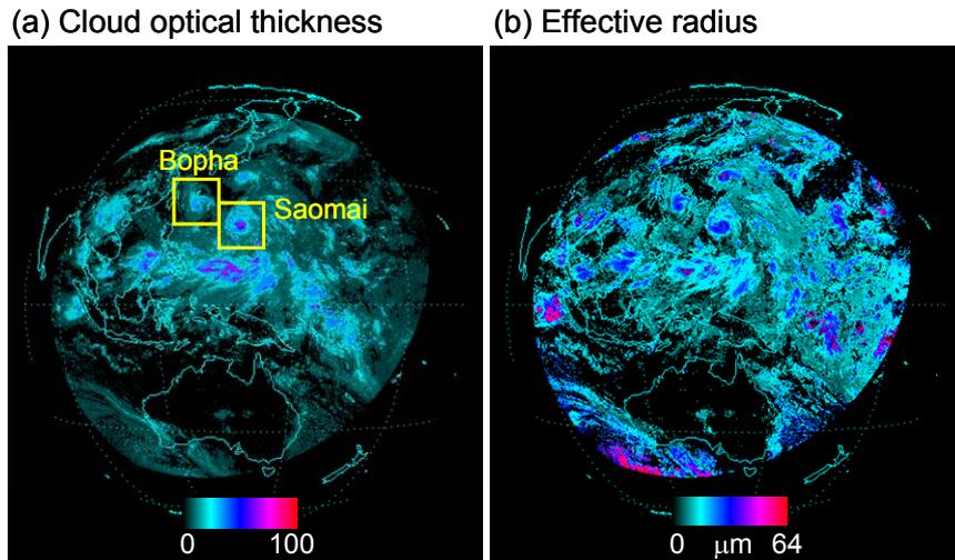
Figure 3 The retrieved cloud optical thickness and effective radius from the MTSAT-1R imagery for 0333 UTC 7 August 2006. Shown are tropical cyclones: Saomai and Bopha centered in 18°N, 139°E, and 23°N, 129°E, respectively.
