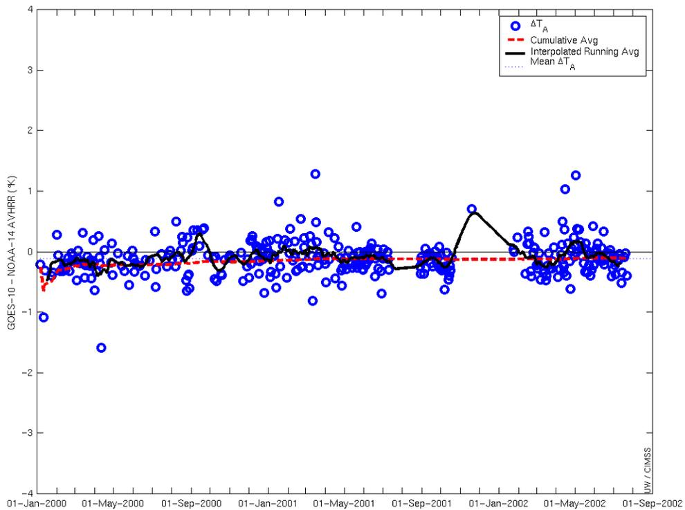
**Figure 6.** Temperature difference time series for GOES-10 and NOAA-14 AVHRR ( $\Delta T_A$ ) in the IRW from January 2000 through July 2002.
