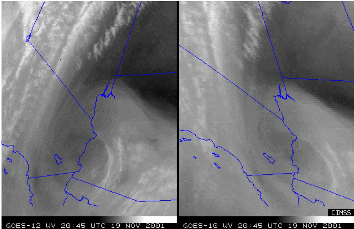
**Figure 3.** The new water vapor channel on GOES-12 (shown here over the western United States) is higher resolution than its predecessors.
