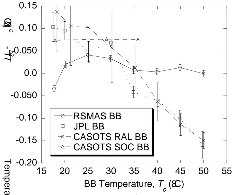
Fig. 6. Comparisons are brightness temperature. The symbols are from the mean values of data points averaged over the last 100 seconds of each plateau of the temperature setting for each blackbody. The error bars are the standard deviation of the values over this time interval.
