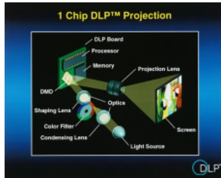
Fig. 2. Digital Light Processor (DLP) projector technology to project appropriate scenes that are radiometrically calibrated using NIST standards.
