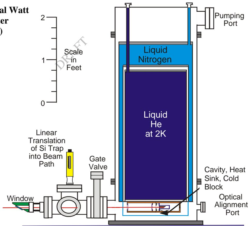
Fig. 3. NIST primary standard for optical power measurements, Primary Optical Watt Radiometer, POWR.
