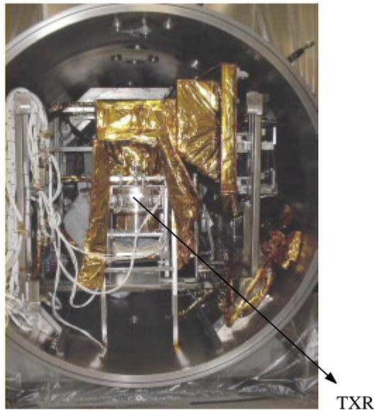
Fig. 7. The TXR in the GOES Imager simulator in the Imager Chamber at ITT. The view is from the back of the TXR. The ECT and SCT sources are located in front of the TXR and so are blocked by the simulator in this view (picture provided by ITT).
