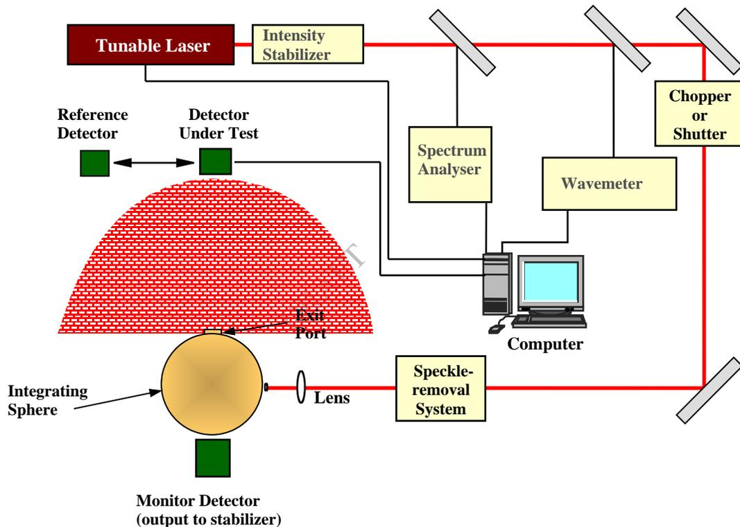
Fig. 4. Spectral Irradiance and Radiance Responsivity Calibrations using Uniform Sources (SIRCUS) Facility at NIST
