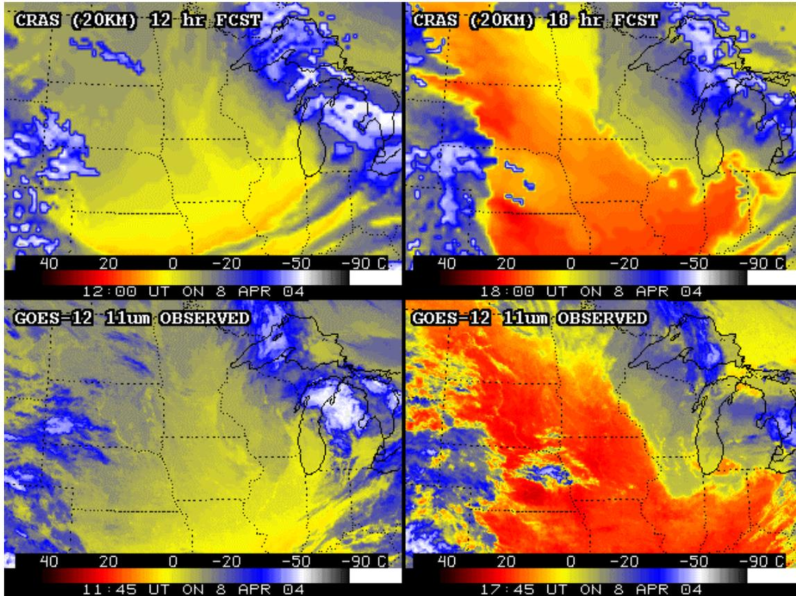
**Figure 9.** Forward calculations from a regional model compared against those from the GOES Imager. Note the fair correlation for cloud cover for both the 12 and 18 hr forecast times.
