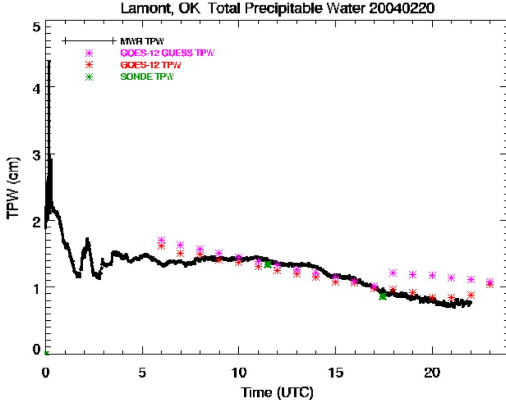
**Figure 1.** GOES-12 sounder TPW validations with a Microwave Radiometer (MWR) at the Department of Energy – Atmospheric Radiation Program (DOE ARM) Southern Great Plains (SGP) Cloud and Radiation Testbed (CART) site. Microwave radiometer (solid line), numerical model forecast (diamonds), rawinsonde measurement (asterisks) and GOES-12 physical retrieval (plus symbols) of total precipitable water vapor value are compared near Lamont, Oklahoma on 20 February 2004 are plotted.
