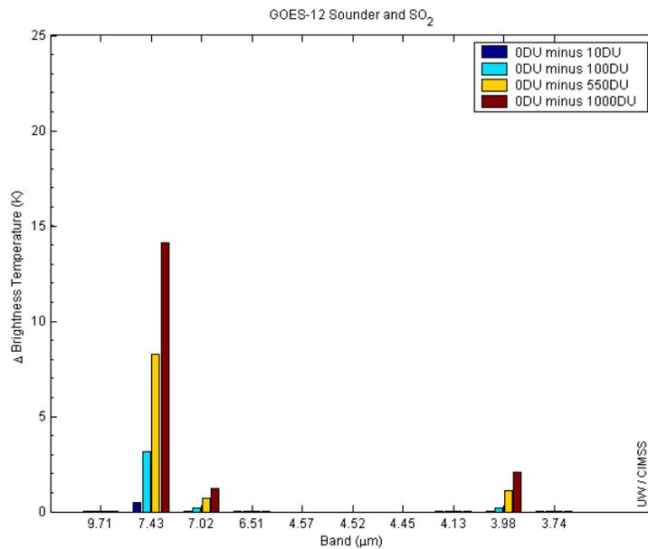
**Figure 8.** Forward calculations showing the brightness temperature impact of SO<sub>2</sub> on several bands on the GOES Sounder. The bar graph is the brightness temperature differences between a simulated atmosphere with no SO<sub>2</sub> and atmospheres of varying amounts of SO<sub>2</sub>.
