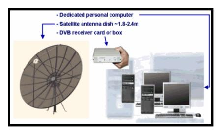
Fig. 3. Components of a typical GEONETCast Americas receiver station.
