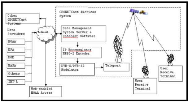
Fig. 2: System architecture illustration.
