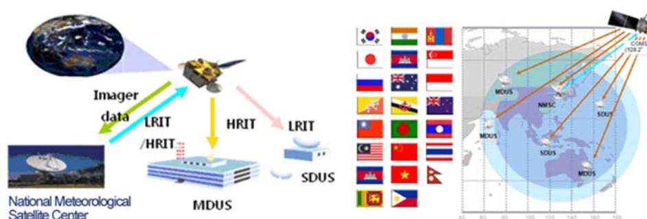
Figure 2.2: Concept of MI H/LRIT direct broadcasting
