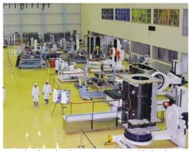
Established in 2006 in a 110 acre campus, ISITE is equipped with state-of-the-art clean room facilities for spacecraft integration and test facilities including a 6.5 Metre thermo vacuum chamber, 29 Ton vibration facility, Compact Antenna Test facility and acoustic test facility under one roof. Assembly, Integration and Testing of all Communication and Navigation Spacecraft is carried out at ISITE. A dedicated facility for the product ionisation of
